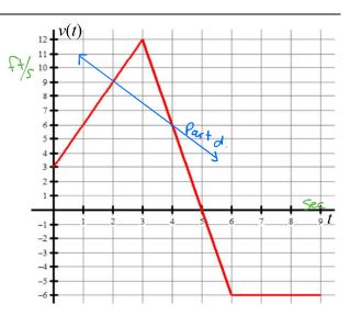
d) What is the average acceleration of the particle over the interval  $2 \le t \le 4$ ? Show the computations and label your answer. Acreleration 15 the rate of change of velocity.
